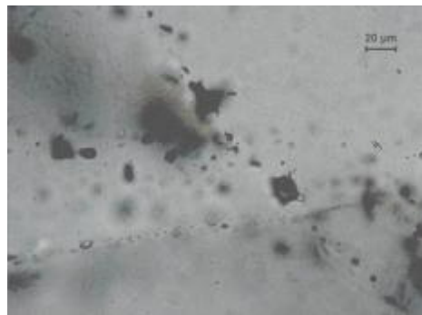
Fig. 3. CO 2 -rich inclusions along late fracture cross cutting CO 2 - H 2 O inclusions in quartz.
